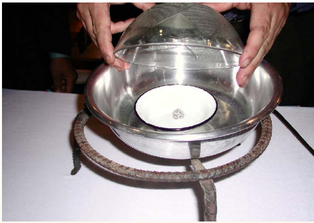
Miners can protect themselves and the environment by using simple kitchen bowl retorts to recover mercury.
